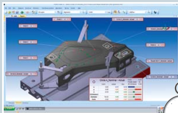
3. Compare measured features to CAD.
